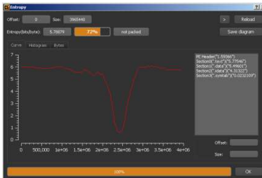
Figure 5 Entropy of the EKANS malware sample. Shows that there aren't any packed sections.
