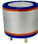
Figure 7: High Gas Concentration Sensors (Bottom is Facing Up)
